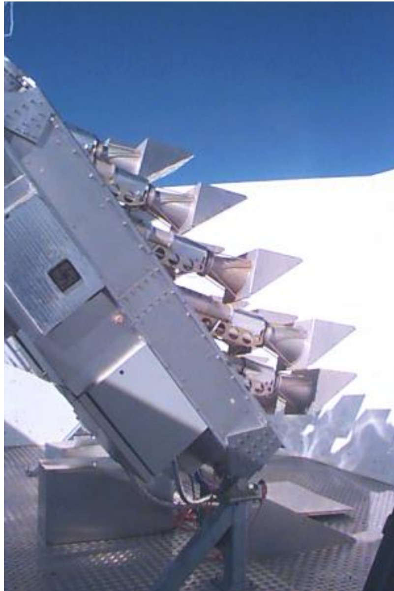
Figure 6.6: VSA showing ground shield
